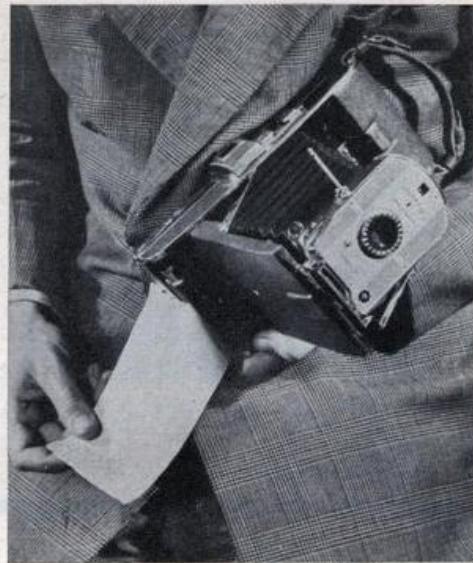
Film is advanced by pulling the leader through slot. Turning a dial in top corner of lens board sets both shutter speed and lens opening.
