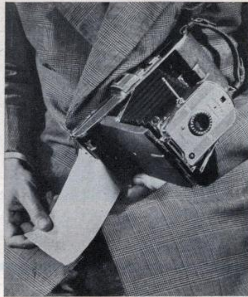
Film is advanced by pulling the leader through slot. Turning a dial in top corner of lens board sets both shutter speed and lens opening.
