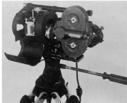
FIG. 5—Bell & Howell 16mm Filmo camera with stereo alternate frame selector. The camera mechanism is coupled with the gear train which drives a 180 degree shutter in front of the beam splitter.
