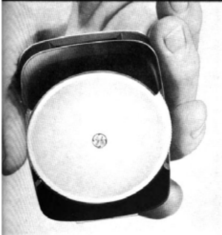
METER ACCURATELY MEASURES color quality of existing light.
