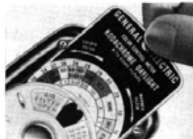
SCALE CARDS adapt meter for popular light sources.
