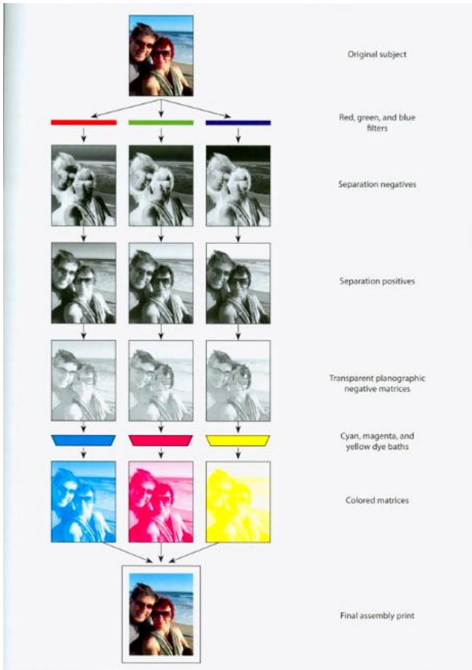
Figure 4.23 Steps of Pinatype printing (planographic matrices).
