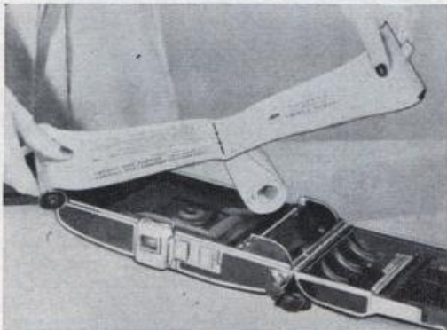
Double film roll drops quickly into loading slots. Positive roll contains eight capsules of developing reagent, one for each print.
